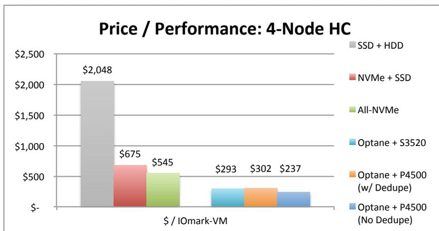
Figure 2: Price / Performance Comparison of Intel Hyperconverged Systems
