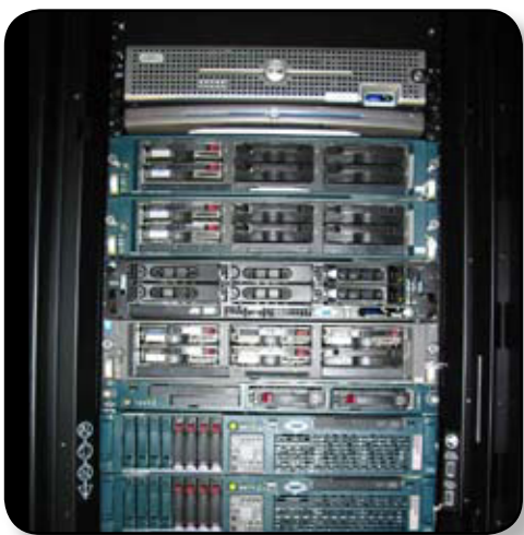
CFCU's call processing, voice messaging, and call center are consolidated in only a few Rack Units (RU) running on Cisco Unified Communications architecture
